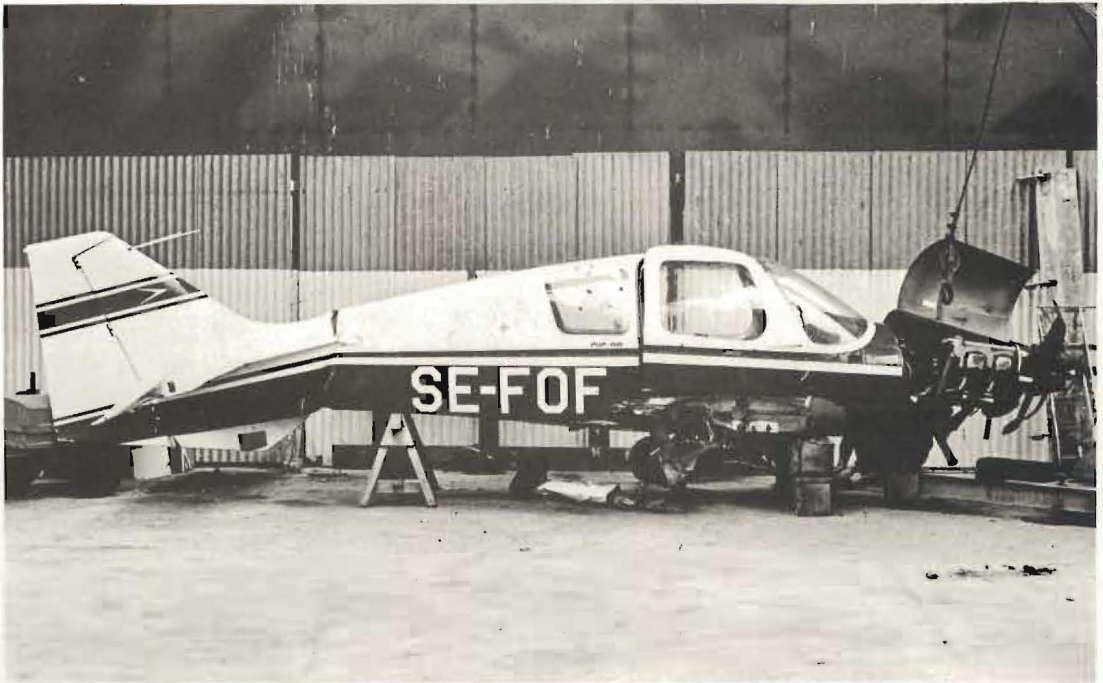
Also at Sywell are the remains of Beagle Pup 150 SE-FOF (c/n B.022) which suffered an engine-failure on approach to the Sywell PFA Rally on July 4th. this year. Luckily, neither pilot nor passenger were hurt.
