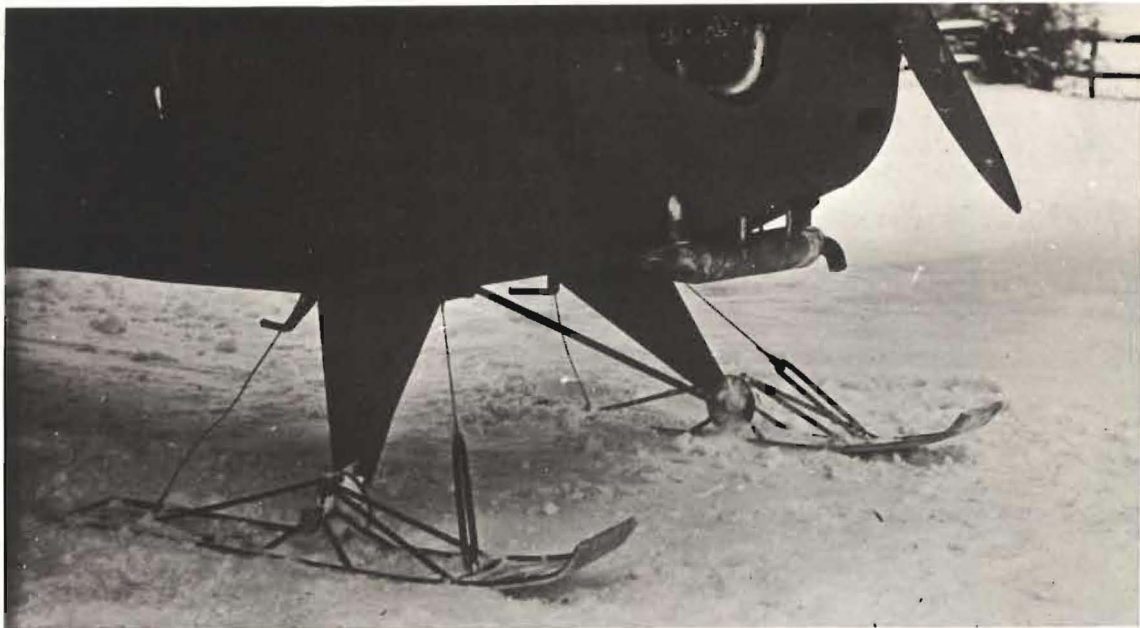
Discovered too late for inclusion in the first issue, is this interesting view of the Model C fitted with skis during January 1940. The obvious crudity of their construction illustrates the fact that they were designed (sic.) made and tested in less than twenty-four hours. (The Mal Sketchley Collection)
